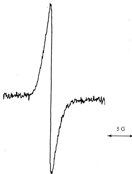
Fig. 1. The EPR spectrum (9.4 GHz) of shortened SWNTs as an aqueous suspension at room temperature.
