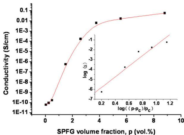
**Fig. 3** –  $\log_{10}$  DC conductivity ( $\sigma$ ) vs. volume fraction ( $p$ ) of graphene/epoxy composites measured at room temperature. Inset:  $\log$ – $\log$  plot for  $\sigma$  vs.  $((p-p_c)/p_c)$  for the same composites. The straight line in the inset is a least-squares fit to the data using Eq. (1). The best fit gave values  $p_c = 0.52$  vol.% and  $\beta = 5.37$  with a correlation factor of 0.97.
