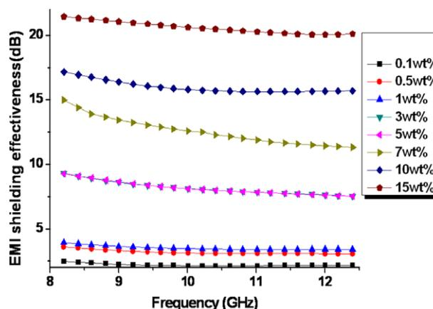
**Fig. 5** – EMI SE of graphene/epoxy composites with various SPFG loadings as a function of frequency in the X-band. The graphene/epoxy composites exhibited SE  $\sim$ 21 dB in the X-band for a 15 wt% loading.
