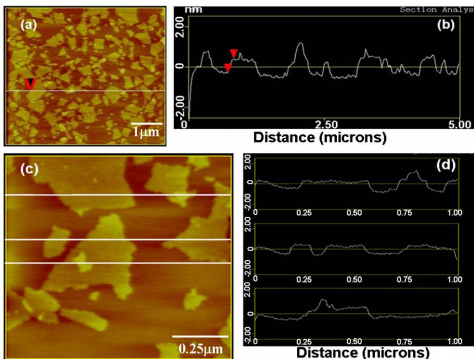
Fig. 1 – (a) A typical tapping mode AFM image of many individual single-layered SPFG sheets deposited on a mica substrate. (b) The corresponding height cross-section along the line in panel (a); the height difference between red arrows is ~0.8 nm. (c) A typical enlarged AFM image of several SPFG sheets deposited on a mica surface. (d) The corresponding height cross-section along the three lines in panel (c).
