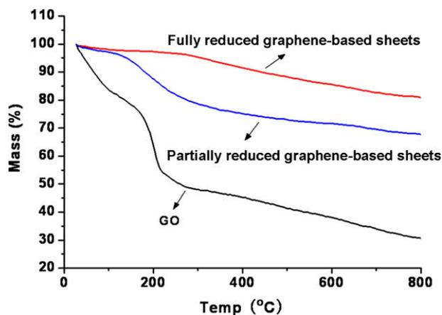
Fig. 2 – The TGA curves with heating rate of 5 °C/min from room temperature to 800 °C under N<sub>2</sub> for GO, partially reduced graphene-based sheets and fully reduced graphene-based sheets.
