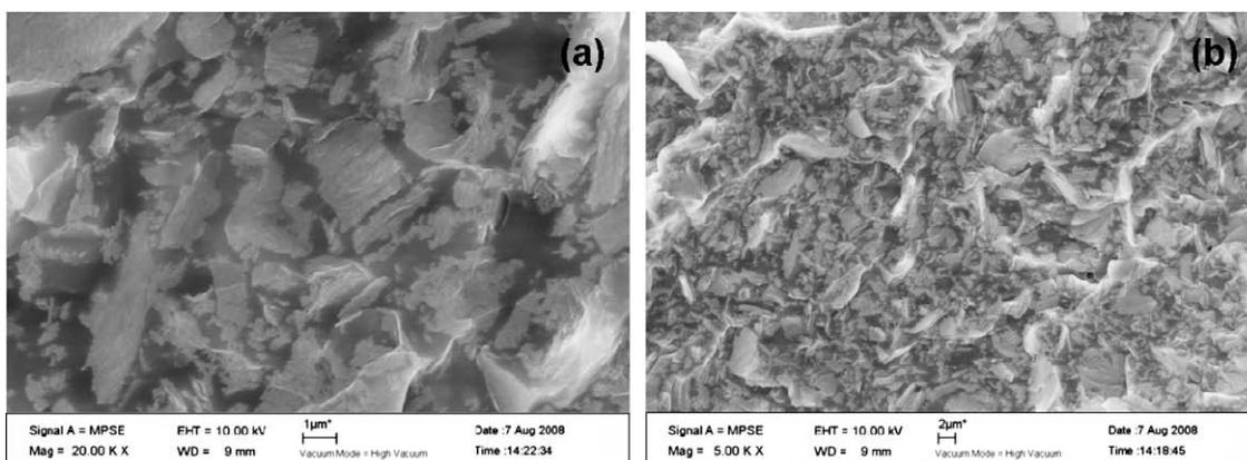
**Fig. 4** – Representative SEM images with two different resolution magnitudes for the cross-section of graphene/epoxy composites with 7 wt% loading of SPFG.
