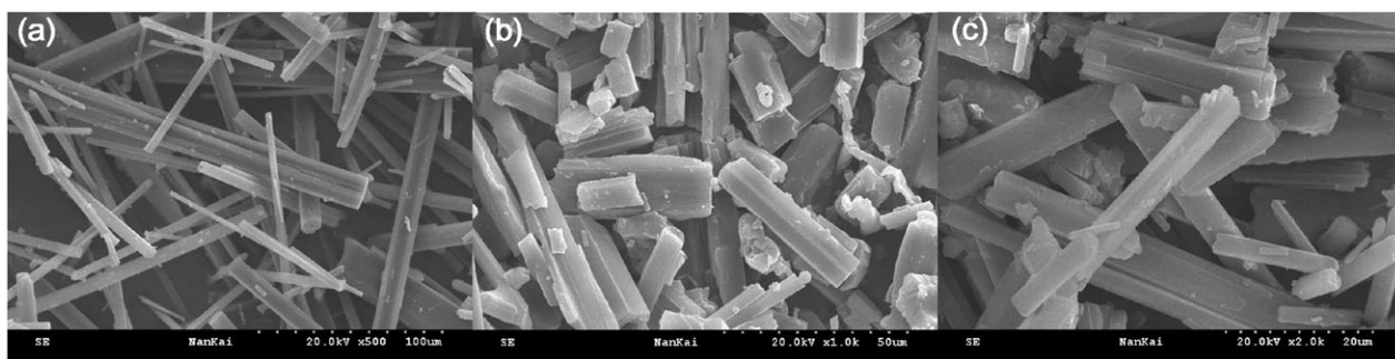
Fig. 7 SEM images of self-assemblies of SA-6 (a), SA-8 (b) and SA-10 (c).
