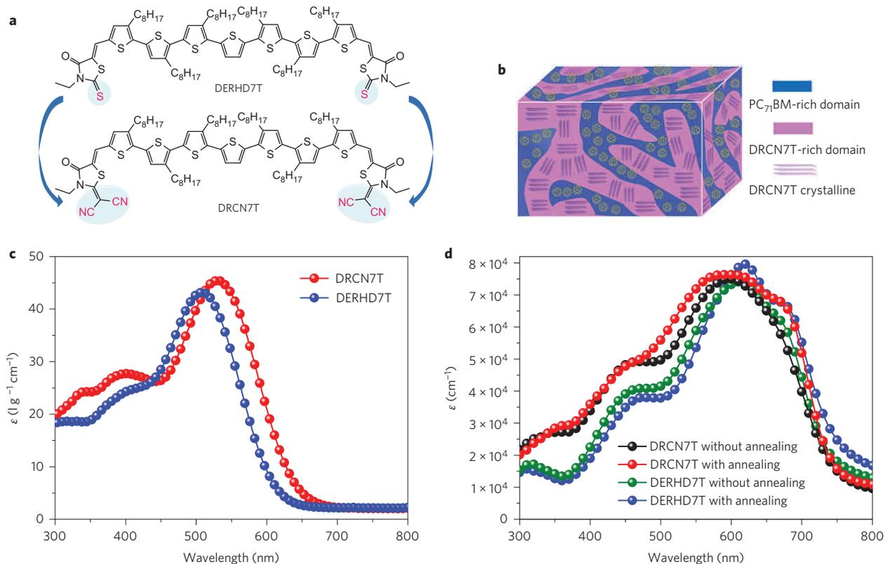
**Figure 1 | Molecular design and characterization.** **a**, Chemical structures of DRCN7T and DERHD7T. **b**, Schematic morphology of the active layer based on DRCN7T:PC<sub>71</sub>BM under optimized conditions. **c**, UV-vis absorption spectra of DRCN7T and DERHD7T in chloroform solution. **d**, UV-vis absorption spectra of neat DRCN7T and DERHD7T films with and without thermal annealing at 90 °C for 10 min.  $\epsilon$  in **c,d** refers to the absorption coefficient.
