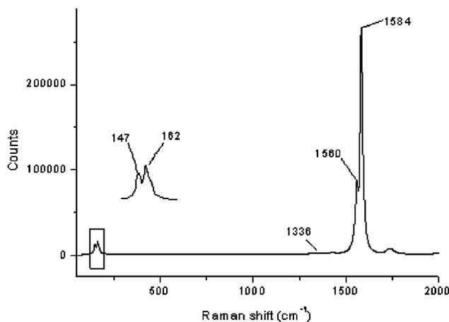
Fig. 1. Raman spectra (excited with 514.5 nm laser) of the web fraction SWNTs obtained using  $\text{NiO-Y}_2\text{O}_3$  as catalyst.
