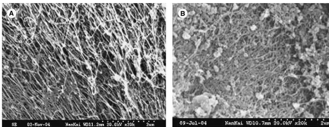
Fig. 2. Typical SEM images of AP SWNTs obtained using  $\text{NiO-Y}_2\text{O}_3$  as catalyst. (A) Web fraction, 20 K, 20 kV. (B) Chamber fraction, 20 K, 20 kV.
