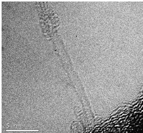
Fig. 3. HRTEM image of AP SWNTs obtained using NiO–Y<sub>2</sub>O<sub>3</sub> as catalyst. Scale bar, 5 nm.
