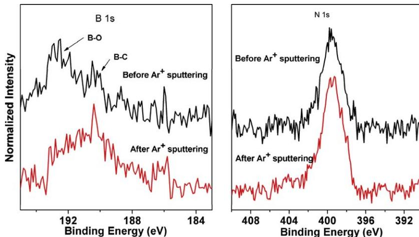
**Fig. 3** – B 1s and N 1s XPS spectra of BN-SWCNTs before (black) and after Ar<sup>+</sup> sputtering (red). The profiles of B–C and N–C bonding inside the bundles are nearly the same as on the surface. (For interpretation of the references to colour in this figure legend, the reader is referred to the web version of this article.)
