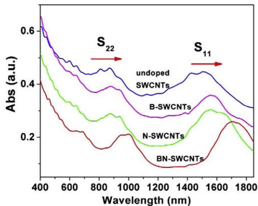
**Fig. 4** – UV–vis–NIR absorption spectra of undoped SWCNTs B-SWCNTs, N-SWCNTs and BN-SWCNTs dispersed in 1 wt% sodium dodecyl benzene sulfonate/D<sub>2</sub>O solution.
