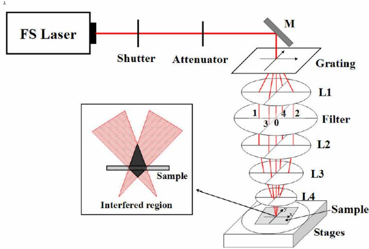
Notes: L1, L2, L3 and L4: lenses; M: mirror; FS Laser: femtosecond laser. The inset shows the overlap of multiplex beams.
