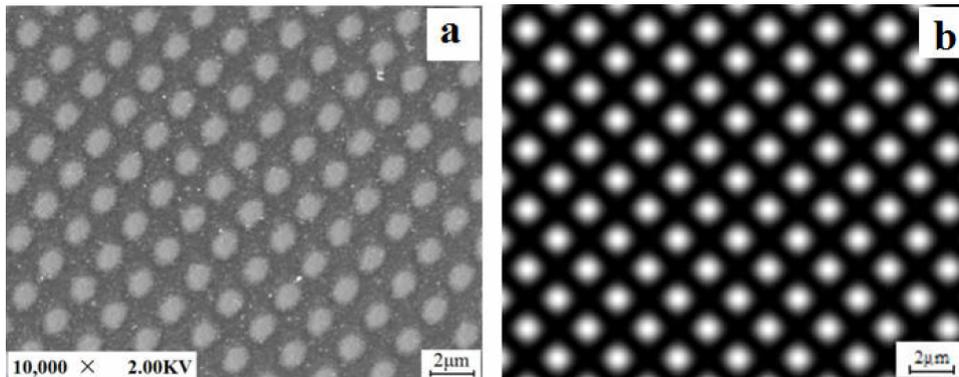
**Figure 5** The square lattice structures on graphene sheet fabricated by 5-beam interference, (a) SEM image of the ablation area (b) the calculated intensity distribution
