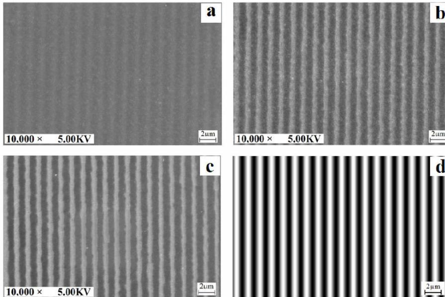
Notes: The distances between the graphene sheet and L4 are (a) 11.5 mm, (b) 12.3 mm, and (c) 13.0 mm, for a compare, (d) shows the simulated intensity distribution of 2-beam interference.
