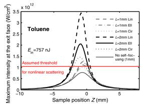
Fig. 8. (Color online) Calculated maximum intensity at the exit face of sample against position Z for different sample length and polarization state.
