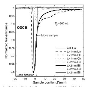
Fig. 9. Polarized light OA Z-scan traces of ODCB at 660 nJ input energy for L = 1 mm and 2 mm (the position of arrow marked by "Move sample" is where we laterally moved the sample at the plane perpendicular to the light axis).
