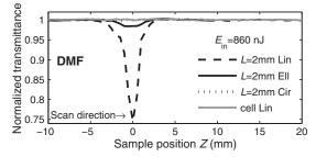
Fig. 10. Polarized light OA Z-scan traces of 2 mm thick DMF at 860 nJ input energy.
