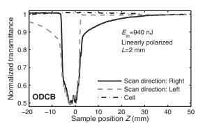
Fig. 11. OA Z-scan traces of ODCB against scanning direction.
