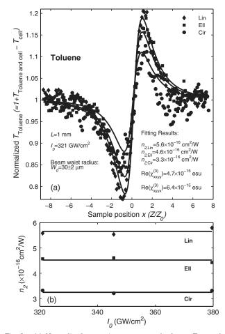
Fig. 3. (a) Normalized transmittance curve of toluene  $T_{\rm toluene}$  for different polarized light at  $I_0 = 321 \ {\rm GW} / {\rm cm}^2$ . (b) Dependence of nonlinear refractive index  $n_2$  on  $I_0$  and polarization state.
