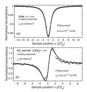
Fig. 1. (a) OA Z-scan trace of 1 mm ZnSe at 800 nm. (b) CA Z-scan trace of  $CS_2$ . The solid lines are theoretical fits, and fitting results are listed in the two figures.
