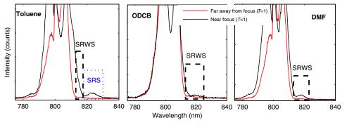
Fig. 6. (Color online) Comparison of forward transmitted light spectra at different sample position.
