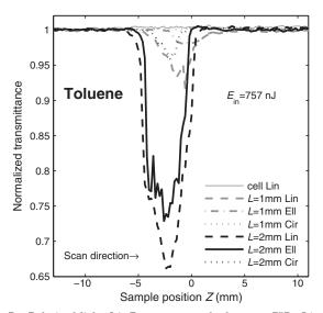
Fig. 7. Polarized light OA Z-scan traces of toluene at 757 nJ input energy for L = 1 mm and 2 mm.
