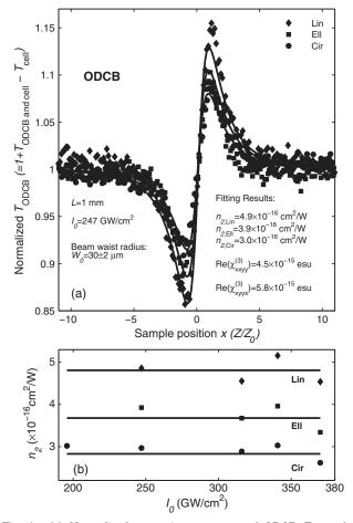
Fig. 4. (a) Normalized transmittance curve of ODCB  $T_{\rm ODCB}$  for different polarization states at  $I_0 = 247 \ {\rm GW/cm^2}$ . (b) Dependence of nonlinear refractive index  $n_2$  on  $I_0$  and polarization state.
