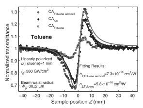
Fig. 2. Linearly polarized light CA Z-scan traces of toluene and cell, quartz cell, and toluene with  $I_0 = 380 \text{ GW}/\text{cm}^2$  and L = 1 mm.
