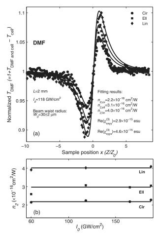
Fig. 5. (a) Normalized transmittance curve of DMF  $T_{\rm DMF}$  for different polarized light at  $I_0 = 118~{\rm GW}/{\rm cm}^2$ . (b) Dependence of nonlinear refractive index  $n_2$  on  $I_0$  and polarization state.
