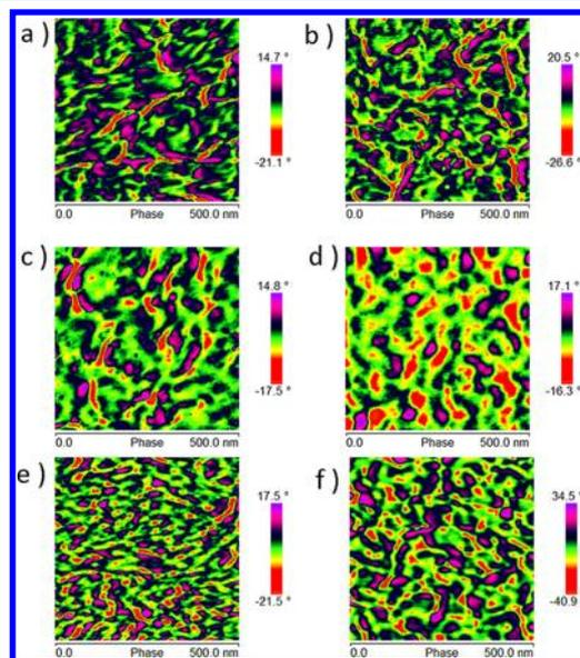
**Figure 3.** Tapping-mode AFM phase images of the active layers of (a, b) DR3TBDTT/PC<sub>71</sub>BM, (c, d) DR3TBDTT-HD/PC<sub>71</sub>BM, and (e, f) DR3TBDT2T (1:0.8 w/w) without (a, c, e) and with (b, d, f) PDMS.
