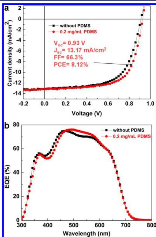
**Figure 2.** (a)  $J$ - $V$  curves and (b) EQE plots for OPV devices based on DR3TBDTT:PC<sub>71</sub>BM (1:0.8 w/w) with (red) and without (black) 0.2 mg mL<sup>-1</sup> PDMS.
