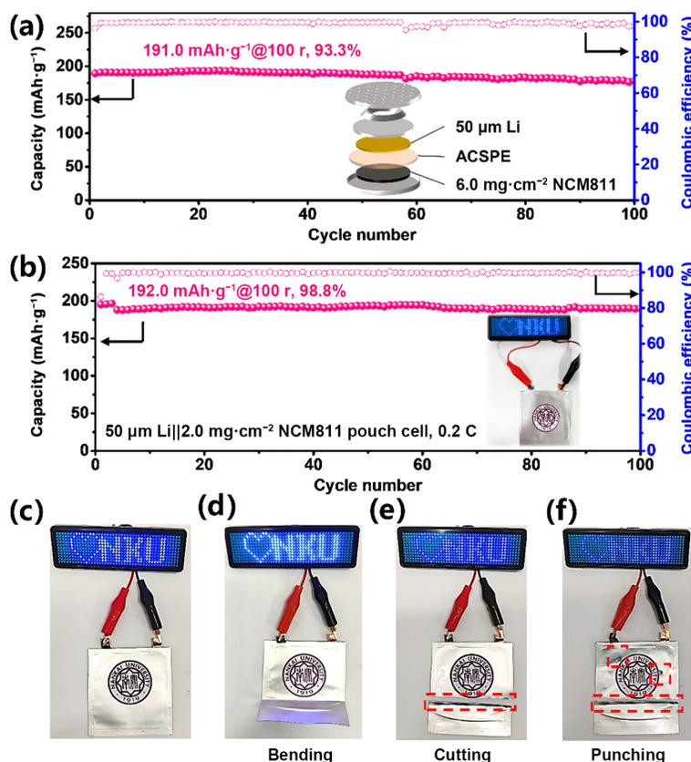
**Figure 4** (a) Cycling performances of  $50 \mu\text{m}$  Li|ACSPE| $6.0 \text{ mg}\cdot\text{cm}^{-2}$  NCM811 coin cell at 0.1 C. (b) Cycling performance of Li|ACSPE|NCM811 pouch cell (inset is optical image of pouch cell powering a light-emitting diode screen). (c) Optical image of a pouch cell powering a light-emitting diode screen and optical images of it under harsh conditions including (d) bending, (e) cutting, and (f) punching.
