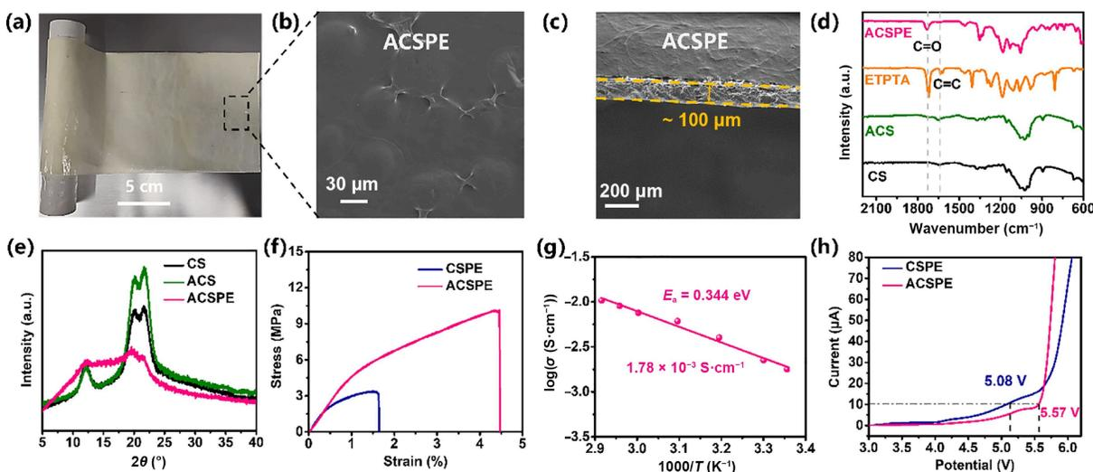
**Figure 1** (a) Digital photograph of ACSPE membrane after UV curing. (b) Surface SEM image of ACSPE membrane. (c) Cross-sectional SEM image of ACSPE. (d) FTIR spectra of CS, ACS, ETPTA, and ACSPE. (e) XRD patterns of CS, ACS, and ACSPE. (f) Stress-strain curves of CSPE and ACSPE membranes. (g) Ionic conductivities of ACSPE at different temperatures. (h) LSV curves of the electrolytes at a scan rate of 1  $\text{mV}\cdot\text{s}^{-1}$  in the voltage range of 3–6 V.
