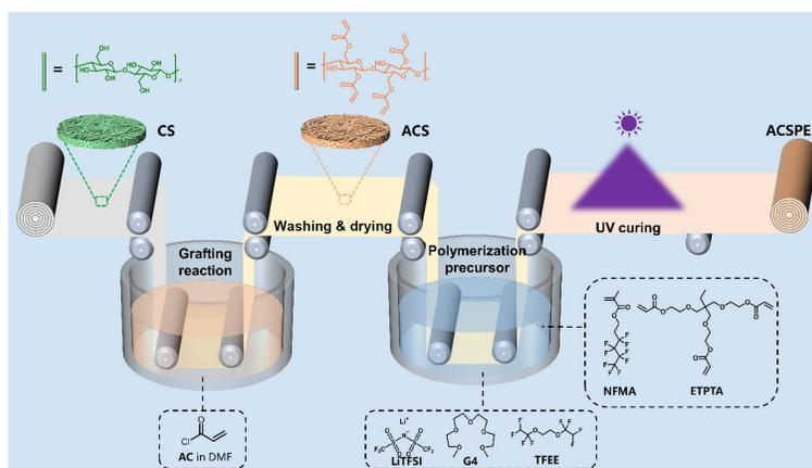
**Scheme 1** Schematic diagram of the roll-to-roll continuous coating fabrication process, which consists of four key steps: grafting reaction, washing and drying, dip-coating with precursor, and UV curing.
