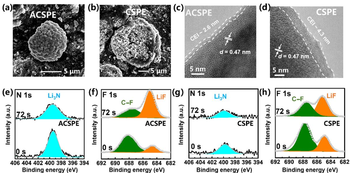
**Figure 5** SEM images of the cycled NCM811 cathodes with (a) ACSPE and (b) CSPE after 50 cycles. TEM images of the cycled NCM811 cathodes with (c) ACSPE and (d) CSPE after 50 cycles. (e)–(h) XPS depth profiles of N 1s and F 1s for cycled NCM811 electrodes with ACSPE and CSPE.
