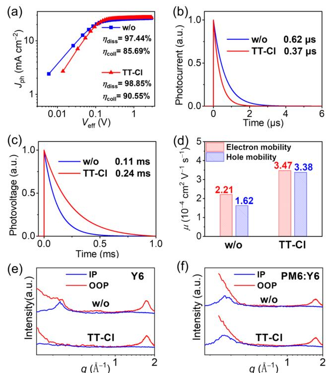
**Figure 3.** (a) Plots of  $J_{ph}$  versus  $V_{eff}$ . The efficiencies of charge generation and collection were also provided. (b) TPV and (c) TPC measurements of OSCs based on PM6:Y6 active layers. (d) Hole and electron mobilities of PM6:Y6-based devices with or without TT-Cl additive. (e,f) 1D line-cuts of Y6 and PM6:Y6-based films with or without TT-Cl additive, respectively, which were derived from their corresponding 2D GIWAXS patterns in Figure S19.
