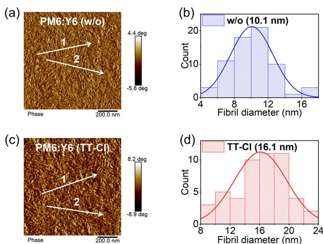
**Figure 4.** (a,c) AFM phase images of PM6:Y6-based films with or without TT-Cl additive, respectively. (b,d) Statistical distribution of fibril width for PM6:Y6-based films with or without TT-Cl additive (see Figure S22 for details).
