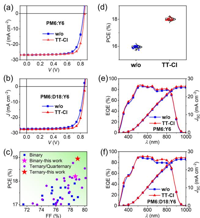
**Figure 2.** (a,b)  $J$ – $V$  curves of OSCs based on PM6:Y6 and PM6:D18:Y6 blends, respectively. (c) A summary of FF and PCE of OSCs based on the widely reported Y6 system (detailed parameters are listed in Tables S14–S15). (d) The performance statistics of OSCs based on the typical PM6:Y6 blends. (e,f) EQE plots of OSCs based on PM6:Y6 and PM6:D18:Y6 blends, respectively.
