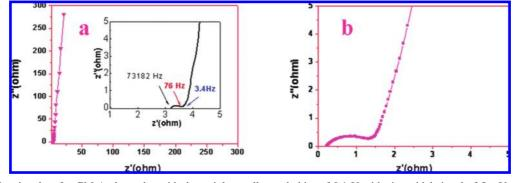
Figure 4. (a) Nyquist plots for GM-A electrodes with the stainless cell at a dc bias of 0.1 V with sinusoidal signal of 5 mV over the frequency range from 100 kHz and 1 mHz. Z': real impedance. Z'': imaginary impedance. Inset shows an enlarged scale. (b) Nyquist plots for GM electrodes without the stainless cell at a dc bias of 0.1 V with sinusoidal signal of 5 mV over the frequency range from 100 kHz and 1 mHz.
