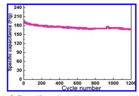
Figure 5. The specific capacitance change at a constant current density of 500 mA/g as a function of cycle number.
