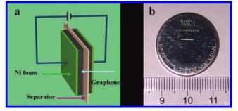
**Figure 1.** Graphene-based supercapacitor device. (a) Schematic diagram of graphene-based supercapacitor device. (b) An optical image of an industry-grade coin-shaped graphene-based supercapacitor device assembled in this study.
