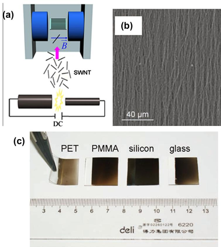
**Fig. 7** – (a) Scheme of fabrication of well-aligned and closely packed SWCNT film on an arbitrary substrate by electric arc discharge with the assistance of a magnetic field. (b) SEM image of aligned SWCNT film obtained by magnetic field assisted electric arc discharge. (c) Photograph of aligned SWCNT films deposited on PET, PMMA, silicon wafer, and glass substrates. Source: Reproduced from [107]. Copyright (2010), with permission from Wiley-VCH Verlag GmbH & Co. KGaA.
