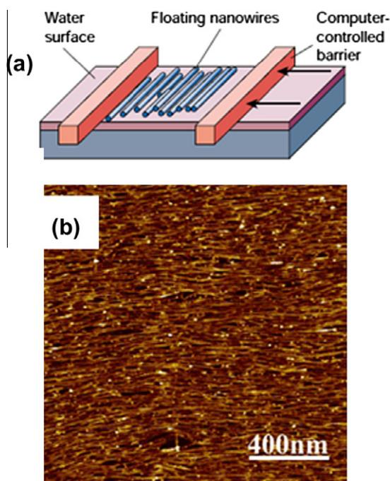
**Fig. 4 – (a) Scheme of Langmuir–Blodgett alignment process. (b) AFM image of a LB monolayer of aligned SWCNTs. Source: (a): Reproduced with permission from [68] Copyright 2003 Nature Publishing Group. (b): Reproduced with permission from [67]. Copyright 2007 American Chemical Society.**
