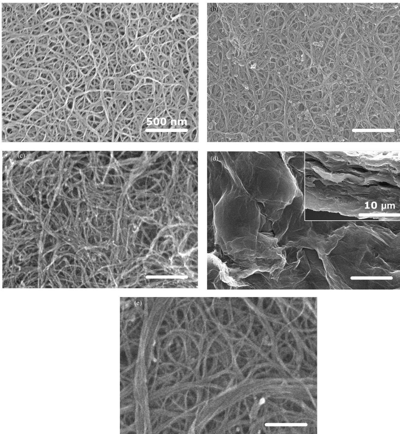
**Figure 7.** SEM images of nanocarbon electrodes, including a) P-SWNT, b) unpurified SWNT, c) P-MWNT, d) RGO and e) P-SWNT/RGO composite (with identical weight percent of both components). The plate-like layered structure of RGO sheets is clearly shown in the inset of Figure 7d.
