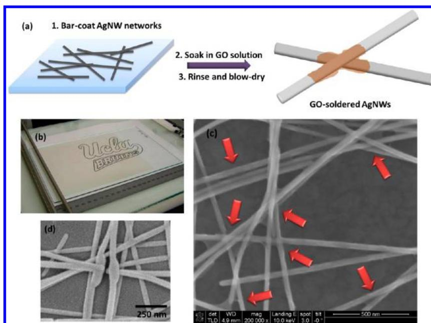
**Figure 1.** (a) Schematic illustration of the fabrication of a GO-AgNW network on a glass substrate at room temperature. (b) Optical photograph of a AgNW network ( $20 \times 15 \text{ cm}^2$ ) bar-coated on a drawdown machine. SEM images of (c) GO-soldered AgNW junctions (indicated by red arrows) and (d) typical high-temperature fused AgNW junctions.
