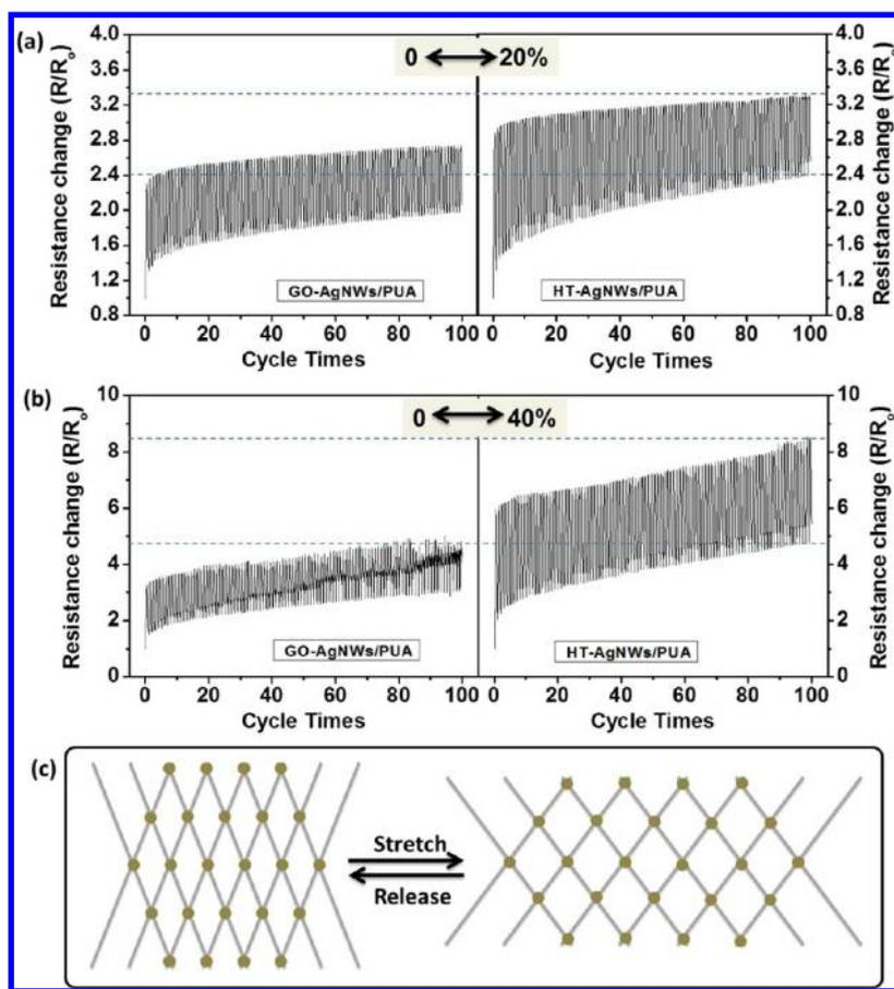
**Figure 6.** Normalized transient resistance of GO-AgNW/PUA and HT-AgNW/PUA composite electrodes during 100 cycles of tensile stretching and releasing between 0 and 20% strains (a) and 0 and 40% strains (b). The initial sheet resistances of both electrodes are 14 ohm/sq. The stretching speed is 1 mm/s. (c) Schematic illustration of the deformation of an ideal nanowire network wherein the nanowire junctions are intact during uniaxial stretching.
