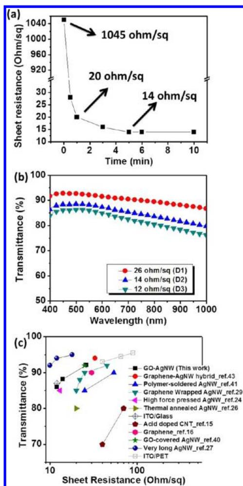
**Figure 2.** (a) Measured sheet resistance of a GO-AgNW network as a function of the soaking time in a GO solution. (b) Transmittance spectra of GO-AgNW networks with three different AgNW densities (D1, D2, and D3). (c) Comparison of the electro-optical performance of the GO-AgNW networks with various TCE films published in the literature and commercial ITO/glass and ITO/PET (all data are exclusive of substrate).
