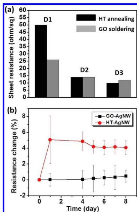
**Figure 3.** (a) Comparison of sheet resistance of GO-AgNW networks with HT-AgNW networks. (b) Plots of the relative sheet resistance change versus time for GO-AgNW networks and HT-AgNW networks with the same AgNW densities (D2) after exposure to hot air (85 °C) for 8 days.
