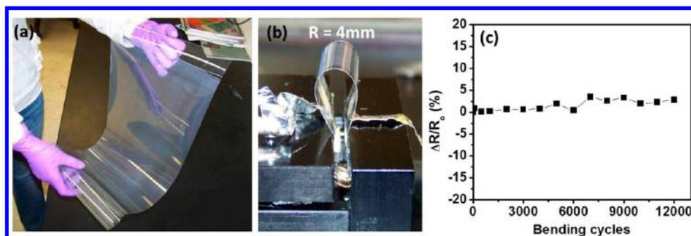
Figure 4. (a) Optical photograph of a GO-AgNW/PET sheet (26 ohm/sq) coated on a drawdown machine (coating area:  $20 \times 40 \text{ cm}^2$ ). (b) Optical photograph of a GO-AgNW/PET bent to 4 mm radius. (c) Relative resistance change of the GO-AgNW/PET during repeated bending–unbending test (bending radius: 4 mm).
