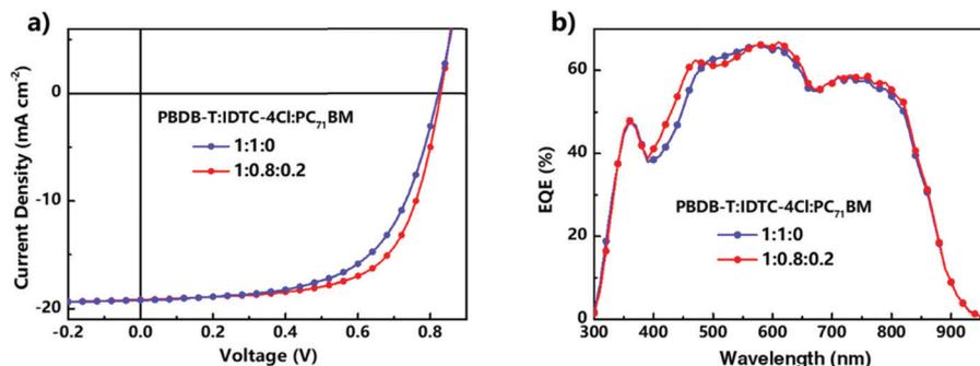
Fig. 4 (a)  $J$ - $V$  and (b) EQE curves based on the binary and ternary devices.
