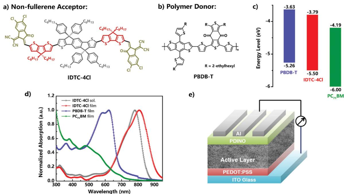
Fig. 1 Chemical structures of (a) **IDTC-4Cl** and (b) **PBDB-T**; (c) energy levels and (d) UV-Vis-NIR absorptions of **PBDB-T**, **IDTC-4Cl** and **PC<sub>71</sub>BM**; (e) the device architecture.
