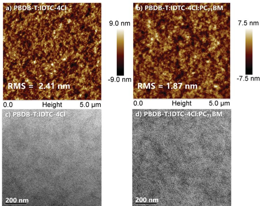
Fig. 6 (a and b) AFM height images and (c and d) TEM images of **IDTC-4Cl** based binary and ternary blends.
