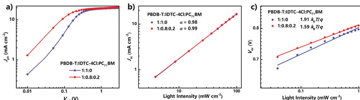
Fig. 5 (a)  $J_{ph}$  versus  $V_{eff}$ , (b) and (c) light-intensity dependence of  $J_{sc}$  and  $V_{oc}$  of their corresponding devices.
