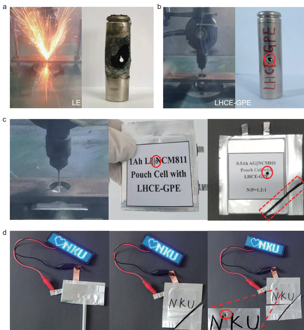
Figure 6. Safety tests of the solid-state polymer electrolyte in various 18650 cylindrical and pouch LMBs. Nail penetration tests of 18650 Li|LE|NCM811 cells (a), solid-state 18650 Li|LHCE-GPE|NCM811 cells (b) and multi-layer Li|LHCE-GPE|NCM811 pouch cells and multi-layer AG|LHCE-GPE|NCM811 pouch cells (c). (d) Safety test of Li|NMC811 pouch cells under various conditions including bending, cutting and punching.
